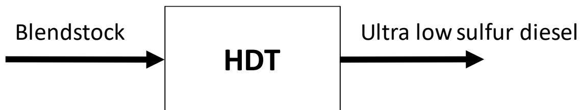
Figure 1 – Reaction section of an ultra low sulfur diesel hydrotreating unit
