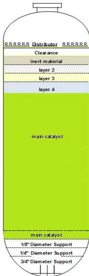
Figure 2 – Illustration of distribution of catalysts and other materials in a reactor of an ultra low sulfur diesel hydrotreating unit
