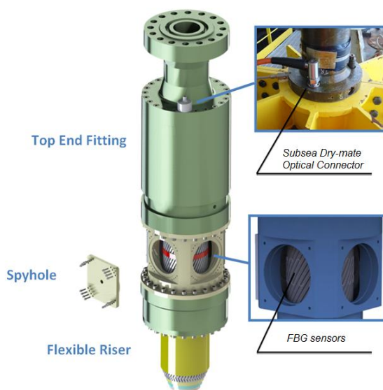
Figure 3: Spyhole End Fitting with MODA sensors
