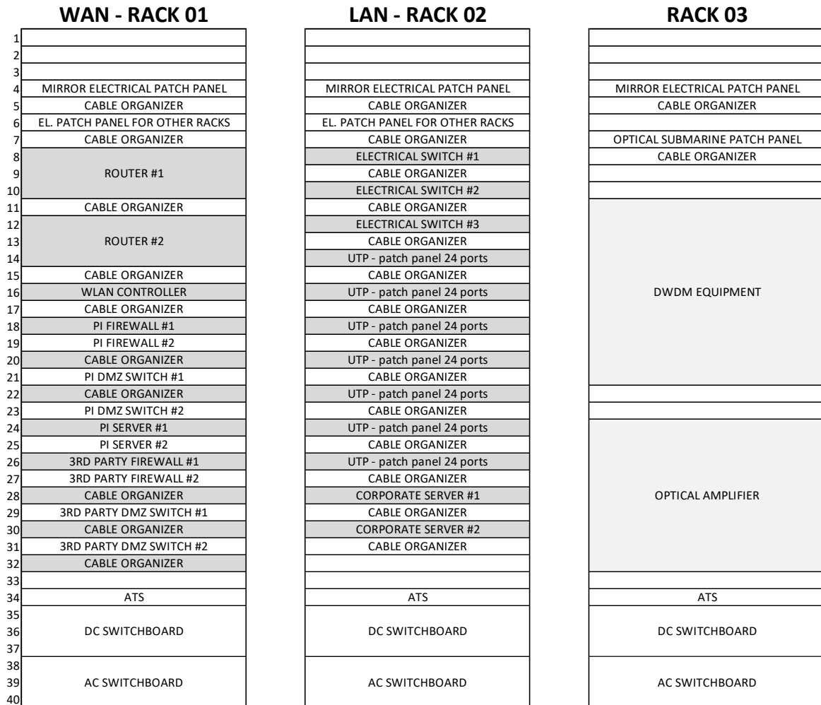
Figure 7: typical layout for PETROBRAS racks
