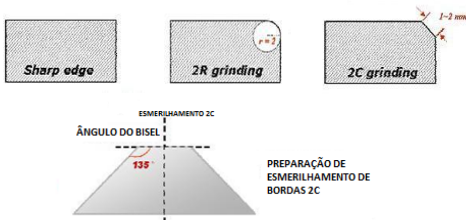
FIGURE 18 -Sharp Edge Preparation Type 2C
