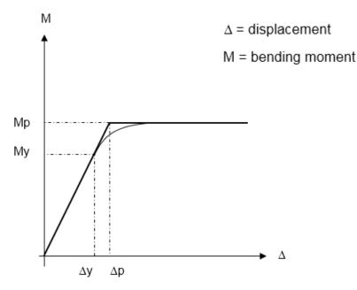
Figure 1 – Material Behavior for Plastic Hinge Analysis
