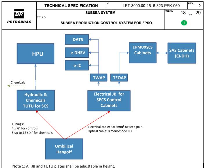
Note 2: All JB and TUTU plates shall be removable to enable the pull in and pull out procedures.
