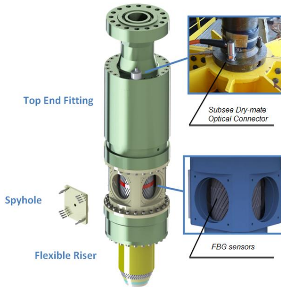
Figure 1 – Spyhole End Fitting with MODA sensors.
