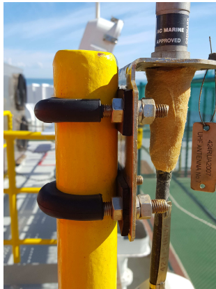
Figure 1: Example of installation to avoid galvanic corrosion
