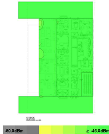
Figure 6: signal strength example on 2.4 GHz band from survey
