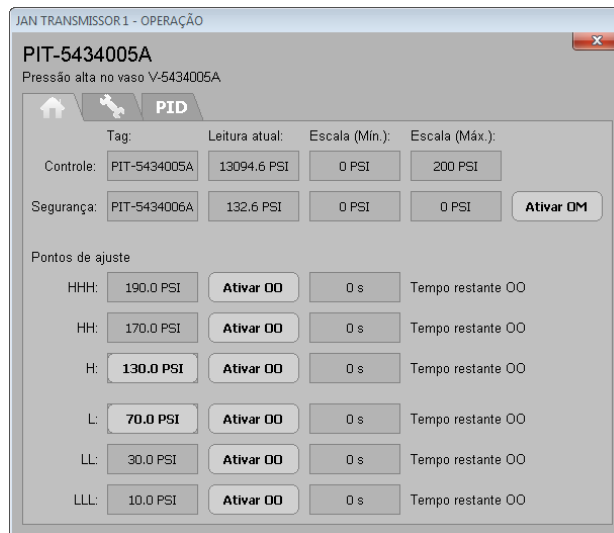
Figure 26 – Example of analog instrument windows operation tab.
