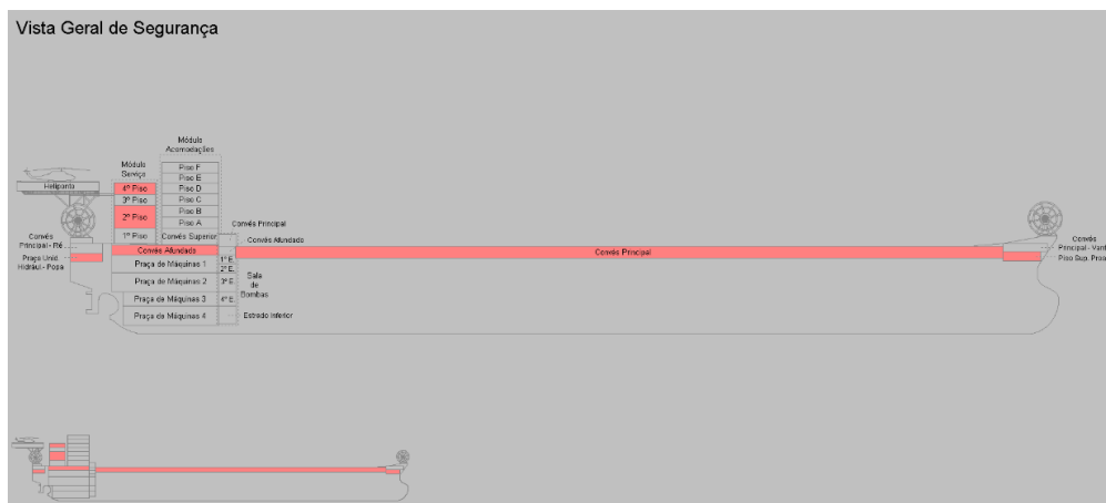
Figure 14 – Example of Safety General View Screen for Hull
