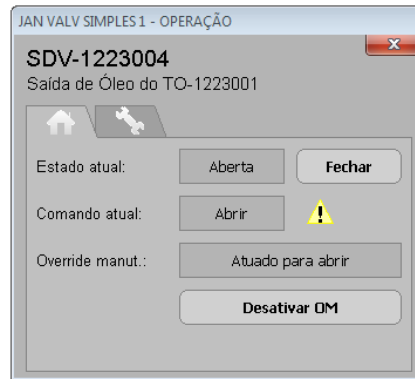
Figure 24 – Example of Command window Operation tab
