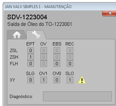
Figure 25 – Example of Equipment command window Maintenance Tab.
