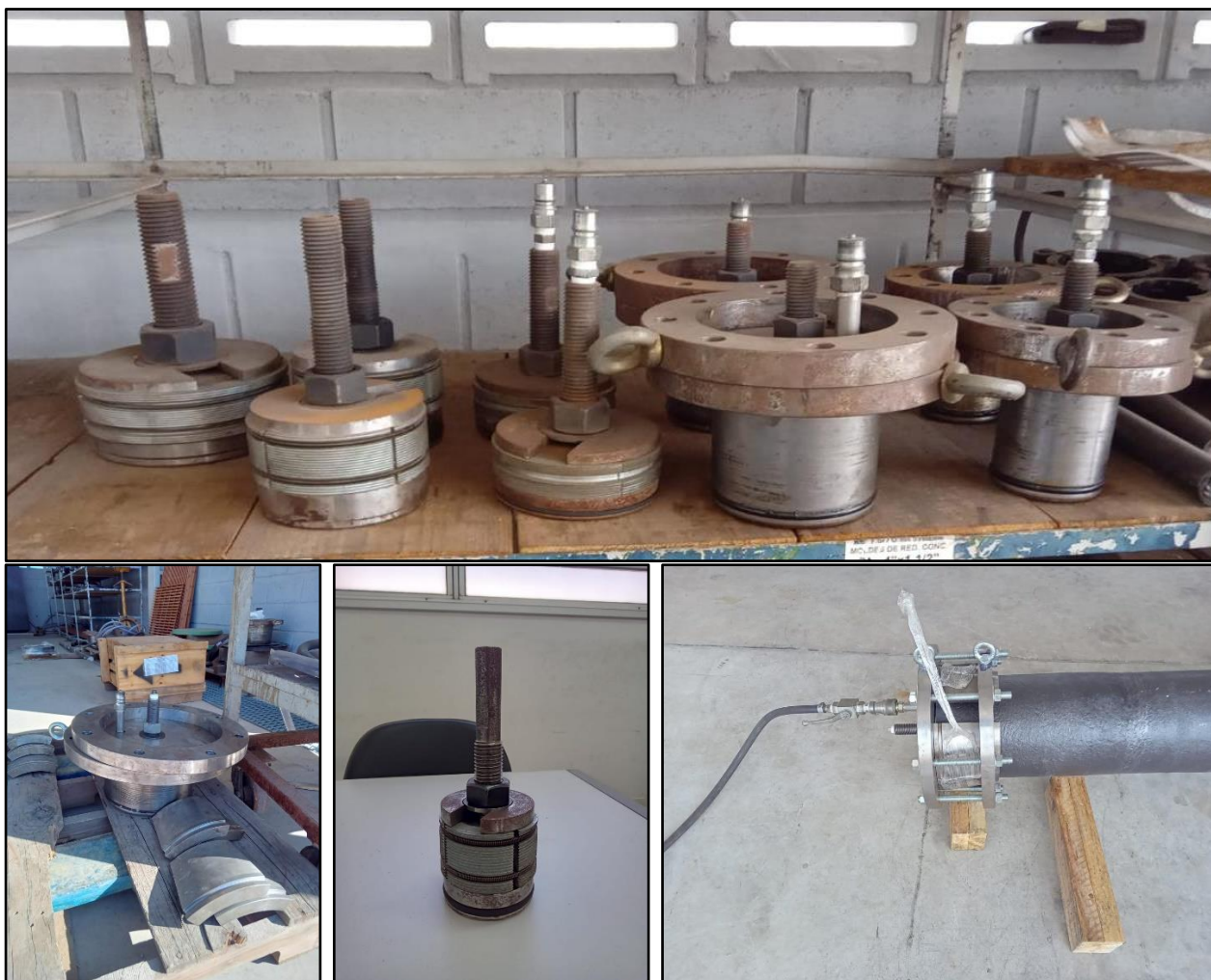
Figure 1 – Examples of plugs for hydrotesting non-flanged end spool pieces.
