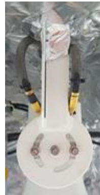
Figure 1: Example of support with azimuthal adjust.
