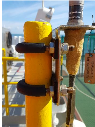
Figure 2: Insulation to avoid galvanic corrosion.
